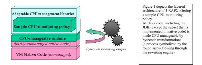
Figure 1. Monitoring using the portable Java CPU management framework.
