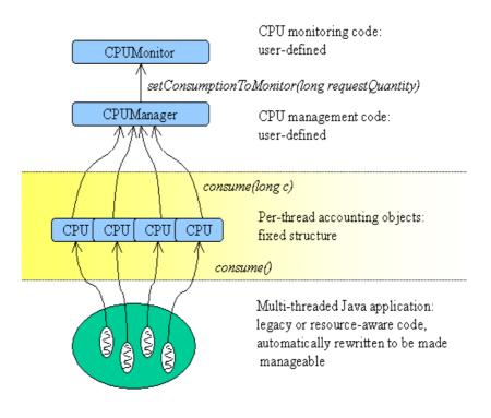
Figure 2. Overview of the CPU monitoring hierarchy.
